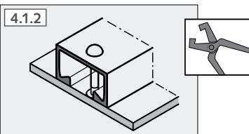
**4.1.2** Fixing using aluminium rivets (supplied by contractor) through the holes in the HALFEN Cast-in channel.
