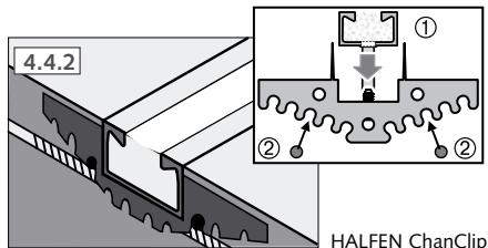
**4.4.2** Fixing from above to the reinforcement, using the HALFEN ChanClip
