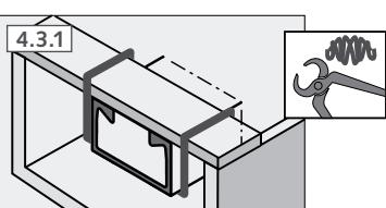
**4.3 Fixing with auxiliary constructions**
