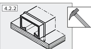
**4.2.2** Fixing HALFEN Channels 28/15 up to 52/34 with staples: Nail the HALFEN Channel to timber form-work with a sufficient number of staples.
